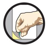
2. Remove white backing tape to expose the sticky resin. Apply patch to repair area with sticky side down and press firmly.
